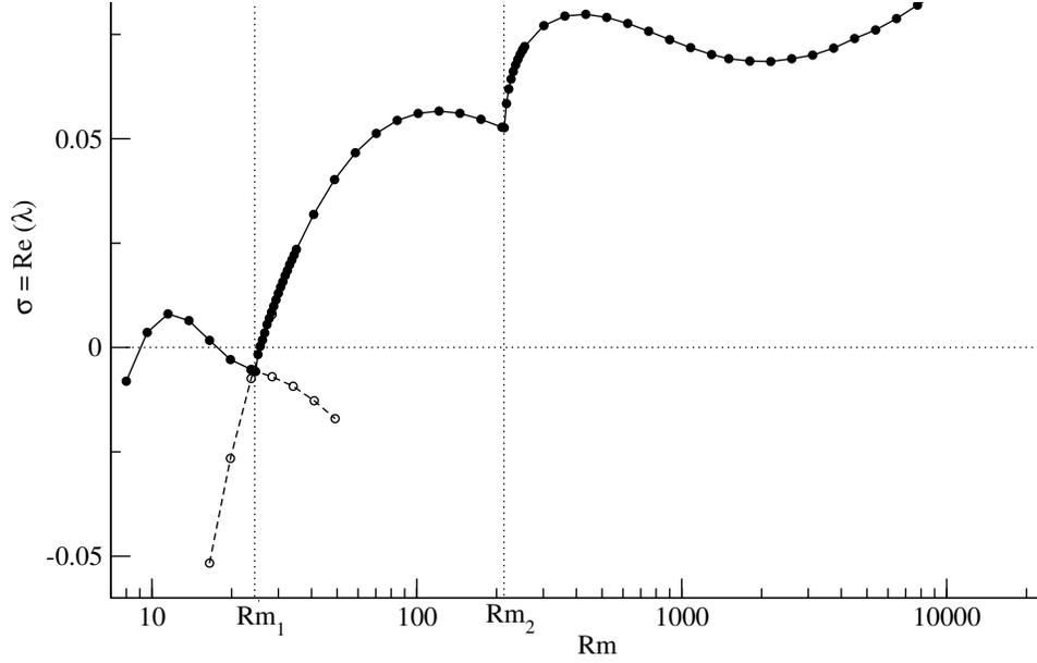
FIG. 1. Plot of the real part of the eigenvalue for the fastest growing magnetic field mode as a function of the magnetic Reynolds number  $Rm$  (using logarithmic scale in the  $x$ -axis).
